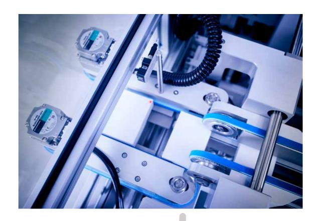
\*Labels in the photographs are red only for demonstration purposes. The real label material is transparent until it is illuminated by the UV light integrated in the system's sensor and will only then glow as red.
